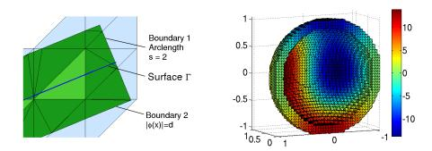
Fig. 6.1. Left: Unfitted narrow-band mesh for a surface with boundary in Experiment 2; Right: Cutaway of a narrow band domain and numerical solution (full active tetrahedra from  $\mathcal{F}_d$  are shown, while integration is performed over cut tetrahedra, i.e. over  $\Omega_h$ ).
