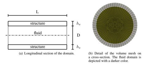
Figure 10. Computational domain for the FSI benchmark.
