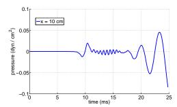
(b) Pressure along the tube centerline
