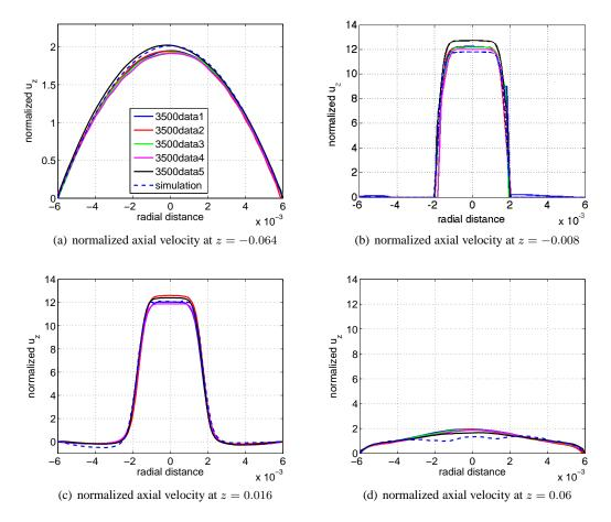
Figure 8. Case  $Re_t=3500$ : comparison between experimental data (solid lines) and numerical results (dashed line) for normalized axial velocity (30) at (a) z=-0.064, (b) z=-0.008, (c) z=0.016, and (d) z=0.06. The legend in (a) is common to all four subfigures.
