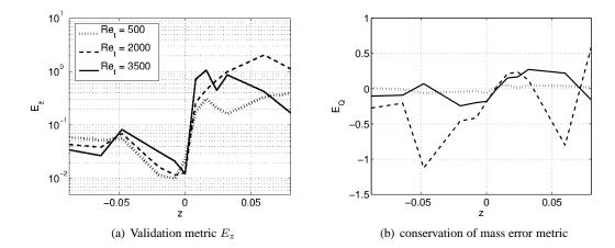
Figure 9. (a) Validation metric  $E_z$  (32) in semi-logarithmic scale and (b) conservation of mass error metric  $E_Q$  (33) as a function of the position along the z axis for  $Re_t = 500, 2000, 3500$ . The legend in (a) is common to both subfigures.
