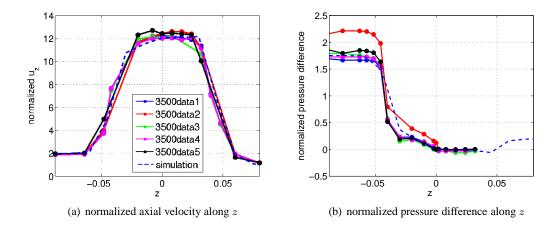
Figure 7. Case  $Re_t = 3500$ : comparison between experimental data (solid lines) and numerical results (dashed line) for (a) normalized axial velocity (30) along the z axis and (b) normalized pressure difference (31) along the z axis. The legend in (a) is common to both subfigures.
