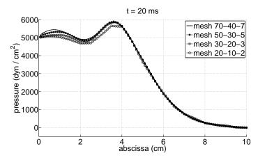
Figure 13. The fluid pressure along the tube centerline at  $t=20\,$  ms, as computed using the four different meshes. The small discrepancies in the computed values show that substantial mesh independence is achieved using the two finest meshes.
