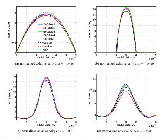
Figure 4. Case  $Re_t=500$ : comparison between experimental data (solid lines) and numerical results (dashed lines) for normalized axial velocity (30) at (a) z=-0.064, (b) z=-0.008, (c) z=0.016, and (d) z=0.06. The legend in (a) is common to all four subfigures.
