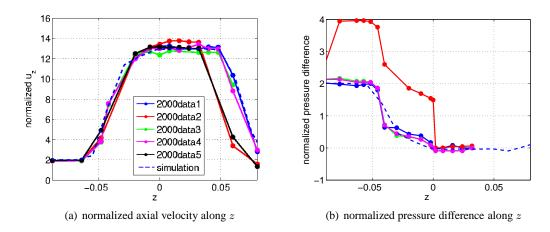
Figure 5. Case  $Re_t = 2000$ : comparison between experimental data (solid lines) and numerical results (dashed line) for (a) normalized axial velocity (30) along the z axis and (b) normalized pressure difference (31) along the z axis. The legend in (a) is common to both subfigures.
