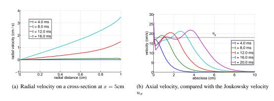
Figure 14. The simulated wave propagation phenomenon matches closely theoretical predictions. Consistently with our assumptions on the model, the radial velocity of the fluid is a linear function of the radial position apart from a thin layer near the tube wall. The fluid velocity on the axis of the pipe approximates the value predicted by Joukowsky's equation. Results obtained on the finest mesh were processed to generate these images.
