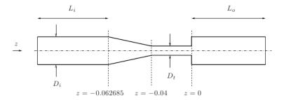
Figure 1. Computational domain. The units are meter.
