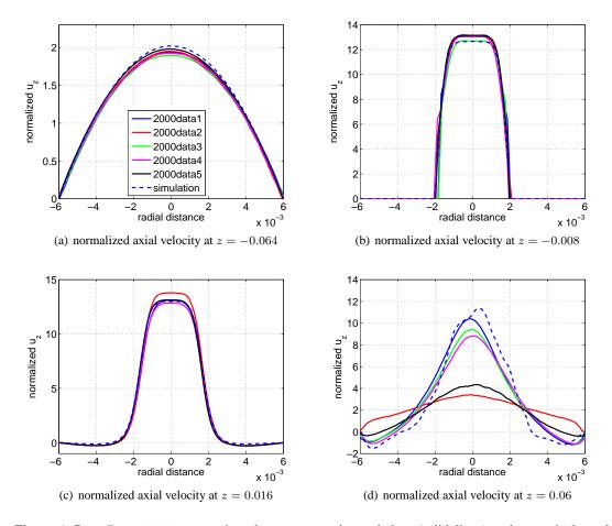
Figure 6. Case  $Re_t = 2000$ : comparison between experimental data (solid lines) and numerical results (dashed line) for normalized axial velocity (30) at (a) z = -0.064, (b) z = -0.008, (c) z = 0.016, and (d) z = 0.06. The legend in (a) is common to all four subfigures.
