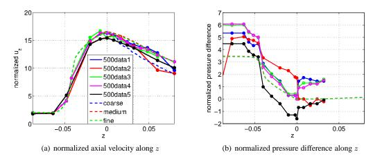
Figure 3. Case  $Re_t = 500$ : comparison between experimental data (solid lines) and numerical results (dashed lines) for (a) normalized axial velocity (30) along the z axis and (b) normalized pressure difference (31) along the z axis. The legend in (a) is common to the two subfigures.
