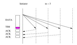
Fig. 2. Illustration of a successful 1-to-m communication
