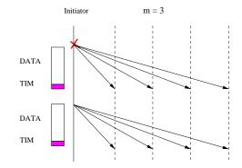
Fig. 4. Illustration of a scenario where the initiator failed to transmit the data message at its network interface. In this case, the initiator needs to retransmit the data frame.
