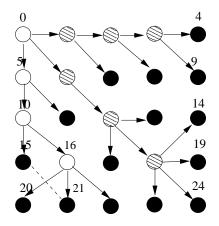
Fig. 9. An instance of Propagation of Information with Feedback. Node 0 fails to determine the termination of procedure although all nodes have received the message. Solid dark nodes are leaf nodes. Nodes that have sent a feedback message to their parents are shaded. The dashed link indicates collision of broadcast messages from node 15.
