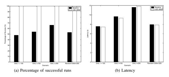
Fig. 10. Propagation of Information with Feedback. Numb. of nodes = 100, wireless transmission range = 250
