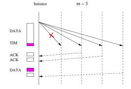
Fig. 3. Illustration of a scenario where some sensors failed to receive the data message. Loss is detected at the initiator. A data frame with no payload is transmitted to solicit further ACKs.
