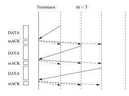
Fig. 5. Illustration of a successful m-to-1 communication where m = 3.
