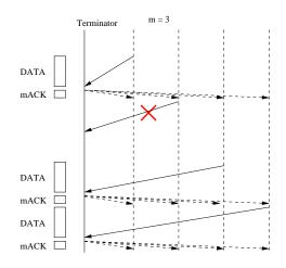
Fig. 6. Transmission from the second node is lost. The remaining nodes need to contend for the channel and re-establish the chain of data/mACK transmissions.
